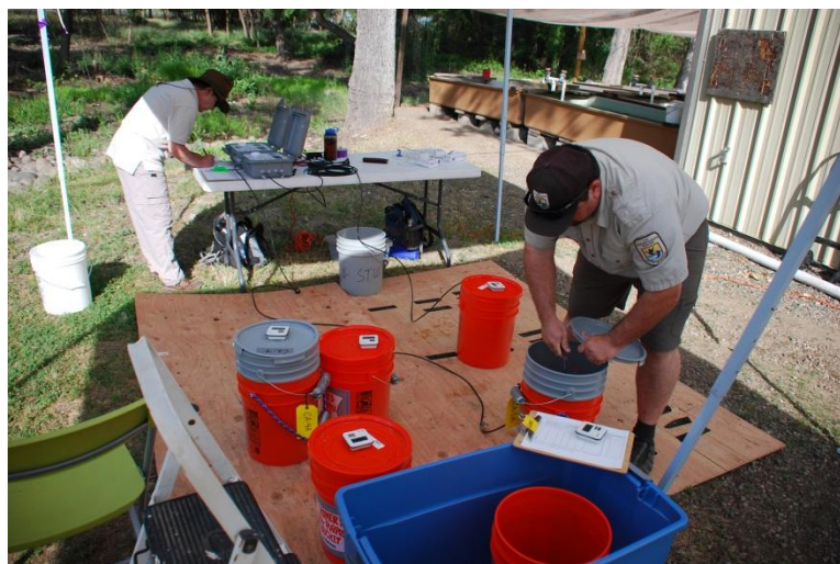
Transmitter verification with VR100 Photo Credit: Ron Smith
