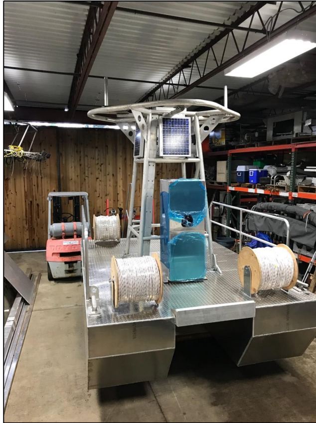
Figure 2: Photograph of pontoon, showing the data tower (sensors not installed), spools for poly-rope, and secure enclosure for instruments, such as data logger and cellular modem.
