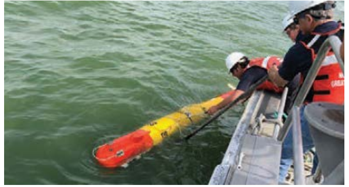
NOAA is using Environmental Sample Processors designed by the Monterey Bay Aquarium Research Institute and mounted on a UUV to study potentially toxic algal blooms in Lake Erie, in collaboration with NOAA's Great Lakes Environmental Research Laboratory.
