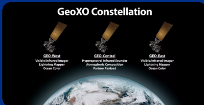
NOAA's Geostationary Extended Observations (GeoXO) satellite system is the ground-breaking mission that will advance Earth observations from geostationary orbit. (Image credit: NOAA/NESDIS)
