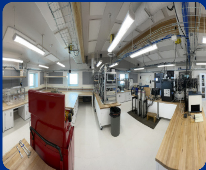
Inside the New Observatory — diverse instruments analyze clean air supplied from the sampling tower. Some instruments measure concentrations of atmospheric gases. Others count and analyze air particles known as aerosols. Records span nearly 50 years, showing long-term trends that would be impossible to discern over a short period. (Image credit: NOAA)
