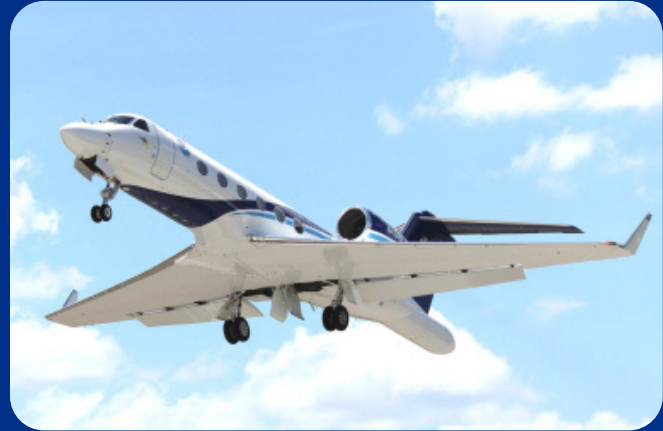
The G-IV is a twin-engine jet piloted by NOAA Corps officers and crewed by NOAA civilian engineers and meteorologists. Its primary mission is to fly tropical cyclone surveillance missions. (Image credit: NOAA)
