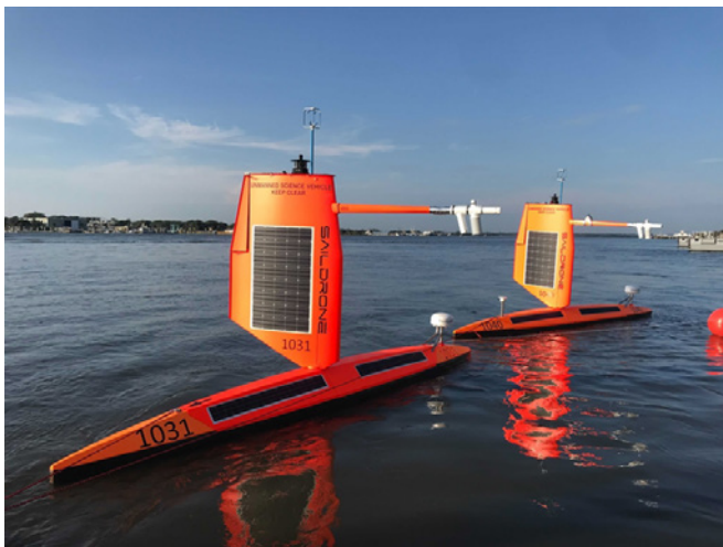
NOAA and Saildrone launched the uncrewed surface vehicles from Jacksonville, Florida at the beginning of the 2021 Hurricane Season to track storms and collect data to improve forecast models. Credit Saildrone
