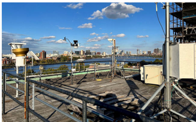
Over the past 8 years samples of methane and carbon dioxide captured at this urban observatory on the roof of a Boston University building have helped scientists show that natural gas leaks from the city are much larger than previously thought. Credit: L.R. Hutyra, Boston University
